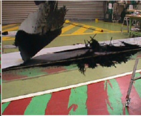
Heavy Damage with Crack, Delamination & Resin Burn-Off – Skin Plies ( 12" x 40" ) Missing – Discharger, Discharger Base & Insert
