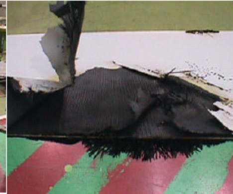
Heavy Damage with Crack, Delamination & Resin Burn-Off – Skin Plies ( 12" x 40" ) Missing – Discharger, Discharger Base & Insert
